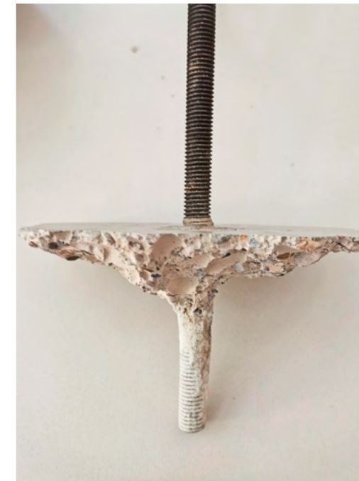
Combined failure of a bonded anchor
